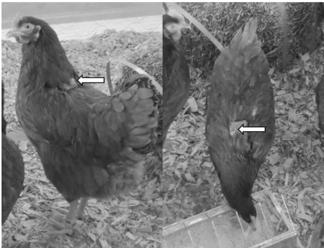
Figure 3 Laying hens fitted with equipment backpacks containing the light monitoring devices used to assess range use. In the picture on the left, the arrow indicates the backpack, in the picture on the right it indicates the top of the light monitoring device sticking out of the wrapping. Photographs were taken in a different study, but the equipment and its attachment were identical.
