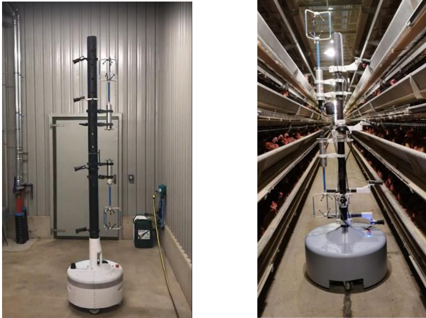
Figure 1: Autonomous navigating robot inside access corridor poultry facility with camera and wind speed sensors fitted (Ross Robotics) and on the right the CAU built platform inside a layer house in Beijing District, China.
