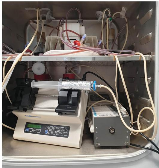
**Fig. 3.** As the dosing syringe is fitted to the HFIM after sterilization it acts as an increased risk of contamination. A syringe filter reduces the risk but is rapidly clogged by MH-F. Dosing with CAMHB overcomes this challenge.
